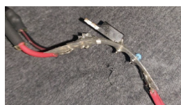
Fig 3. Soldered flexible board with resin protection.
