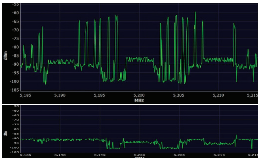
Figure 14. Screen capture of the measured spectrum with S-04 in Rx mode with the LAP-01 and LBM-01 linked (up) and then both switched off (down).
