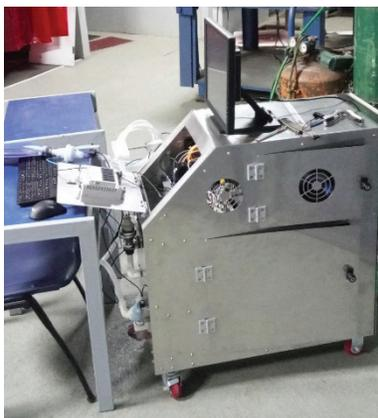
**Figura 1.** Lateral view of the respirator with metal case.
