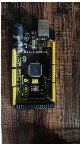
**Figura 3.** Tarjeta Arduino MEGA.
