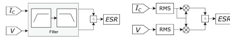
Fig. 2. a) Technique of ohmic frequency range b) Technique for AC power losses
