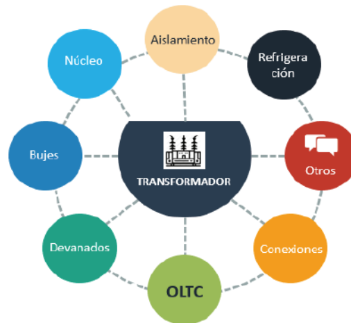
Figura 10. Subcomponentes del transformador de potencia. Fuente. Adaptado de [3] oil reclamation, testing methods for the determination of remaining insulation (paper).
