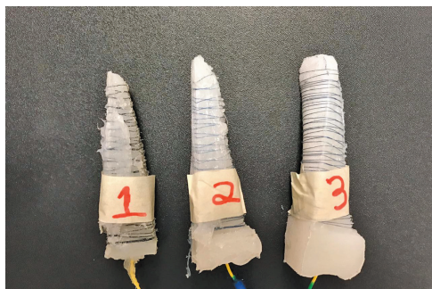
Figure 2. Pneumatic muscles made with different silicones.
