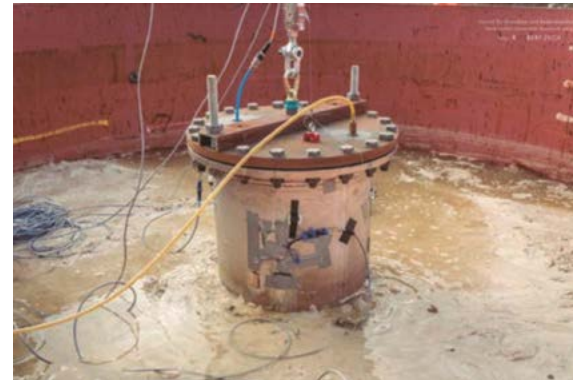
Fig. 1 Decommissioning with overpressure – sealed pile head equipped with pressure and strain sensors
