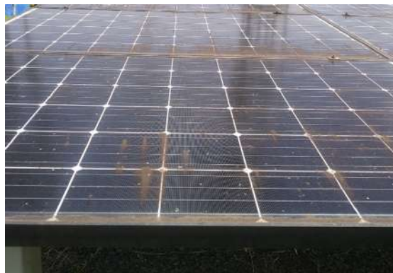
Fig. 2. Soiled PV module.
