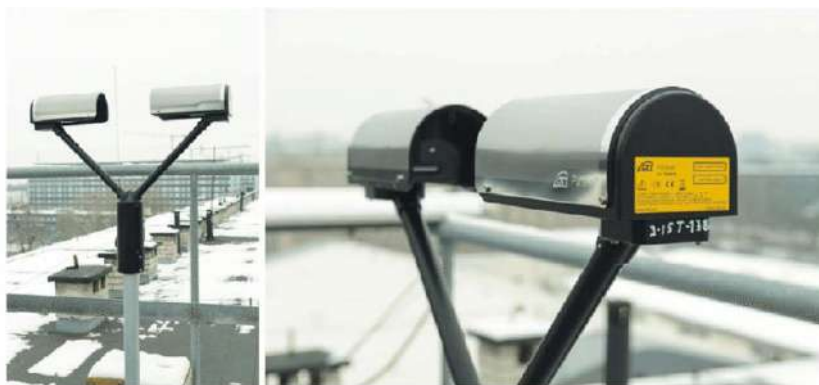
Figure 5. OTT Parsival2 laser disdrometer ( https://www.ott.com/products/meteorological-sensors-26/ott-parsival2-laser-weather-sensor-2392/ ).
