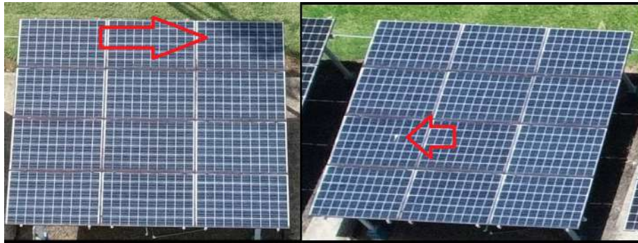
Fig. 1. Partial shadow on a PV panel (left) and strange object on a PV panel (right).
