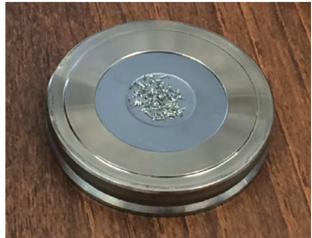
Figure 1. Sample placement on the silicon sample holder for the x-ray diffractometer.
