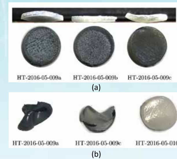
Fig. 1. Deformation presented in samples after exposed to high temperature plasma: (a) PVA substrates, (b) PLA substrates
